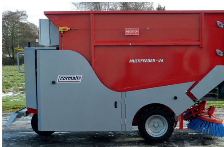
Figure 5: Self-propelled distribution cart (Multifeeder V4) (Source: works photo Cormall)
