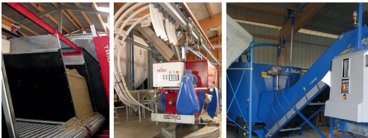
Figure 4: Left: stock container; Middle: rail-mounted mixing and distribution cart; Right: stationary mixer and rail-mounted distribution cart (Source: Oberschätzl)
