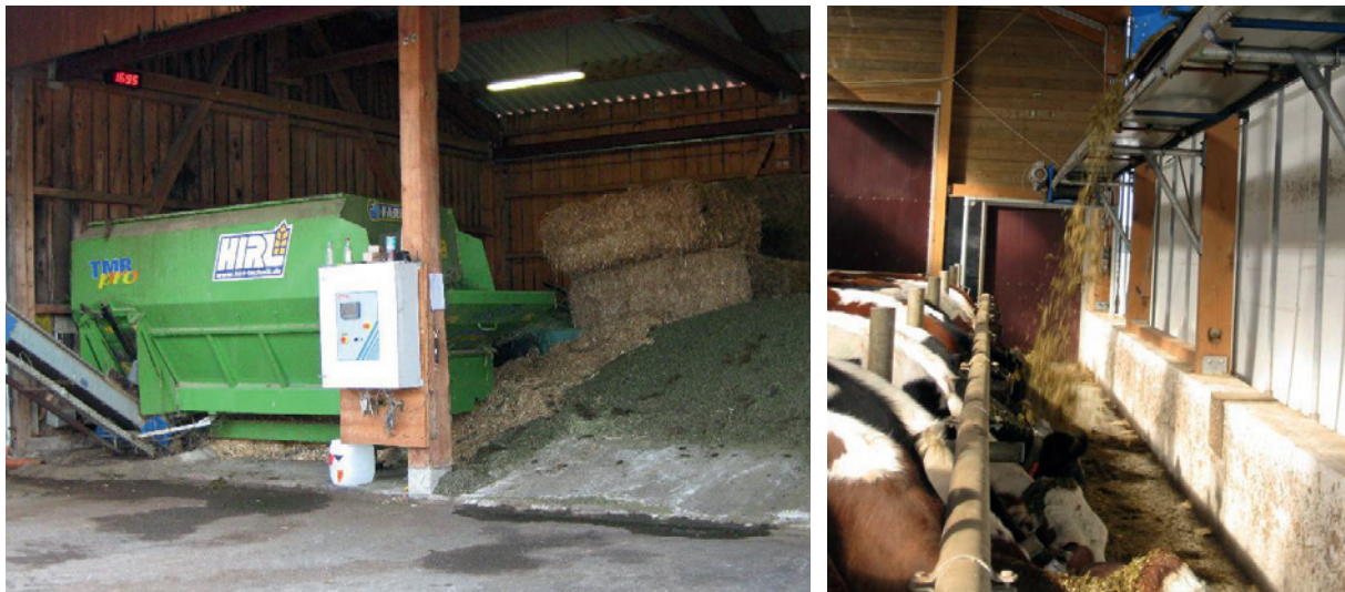
Figure 3: Left: stationary mixer with control unit; Right: conveyor belt mounted over the feed alley (Source: Oberschätzl)
