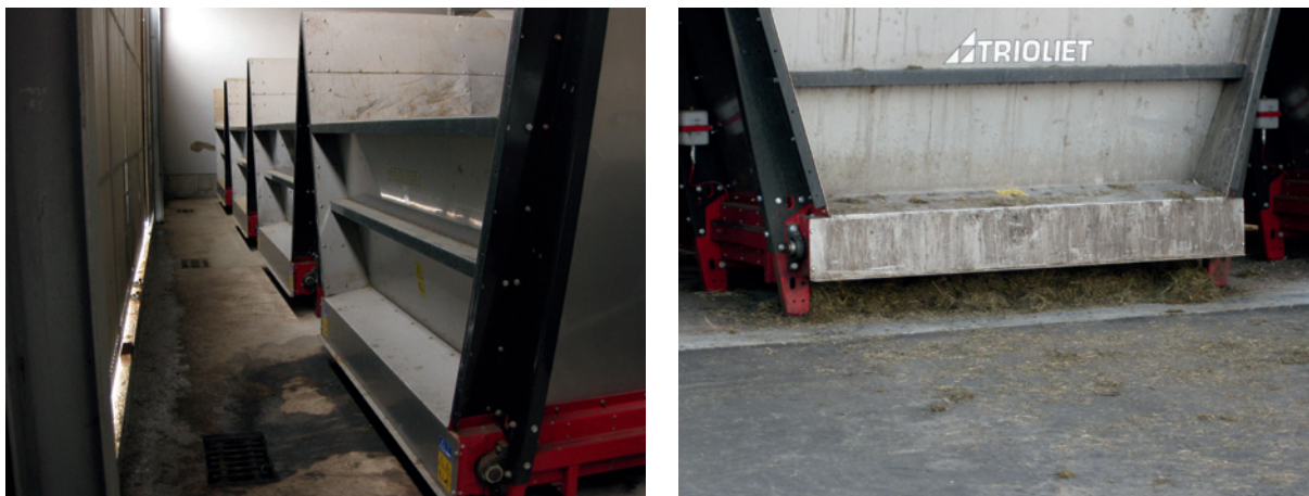
Figure 9: Left: discharge opportunities for cleaning water and silage effluent Right: feed residues at the cleaning flap (Source: Oberschätzl)
