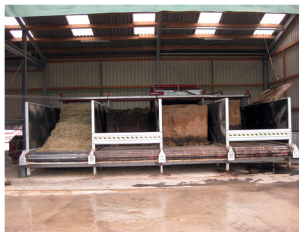
Figure 8: Left: sloping arrangement of stock containers; Right: horizontal position of stock containers (Source: Oberschätzl)
