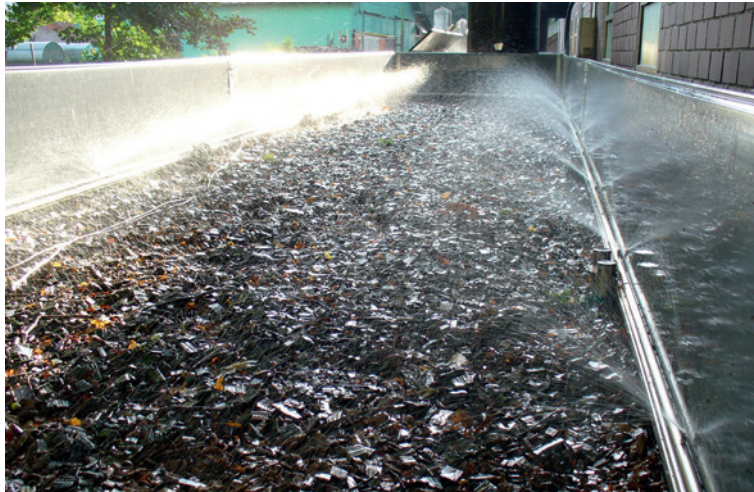
Figure 2: Single-stage biofilter with running trickling (photo Dr. Hahne)
