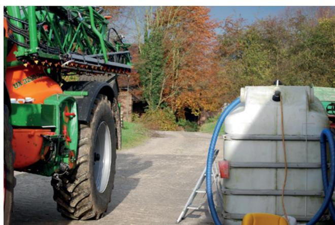
**Figure 3:** Buffer tank for water for filling (source: Kramer)
