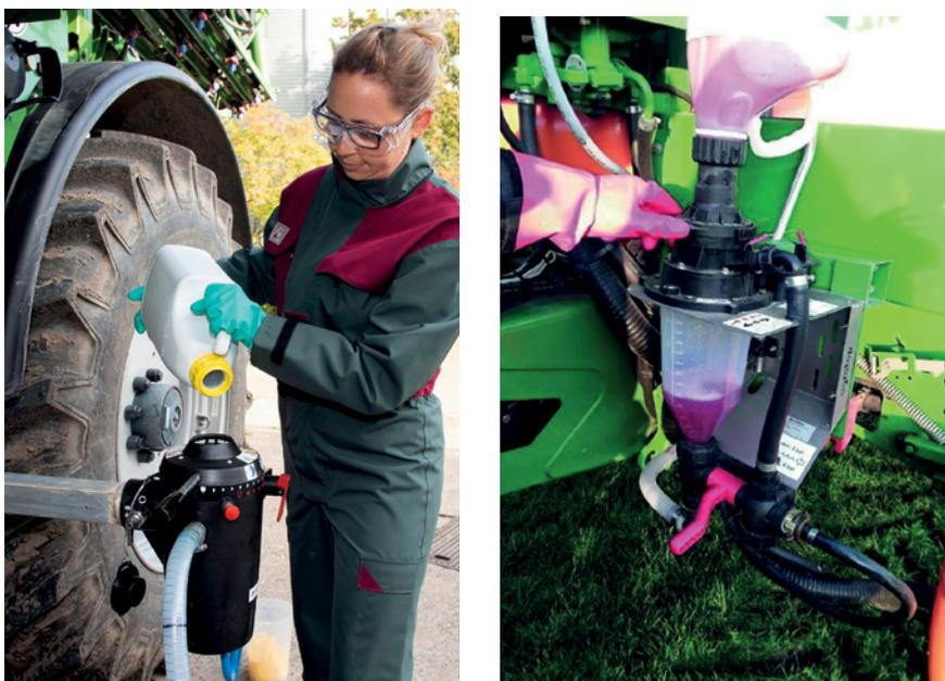
**Figure 6:** Left: BASF EasyConnect (source: BASF SE); right: measurement and partial quantity removal with EasyFlow M (source: Kramer)
