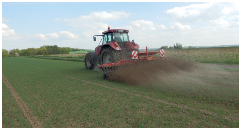
Figure 4: Rotary star hoes are good crust breakers on loamy soils and are suitable additions to tine harrows (source: Markus Mücke, Landwirtschaftskammer Niedersachsen)
