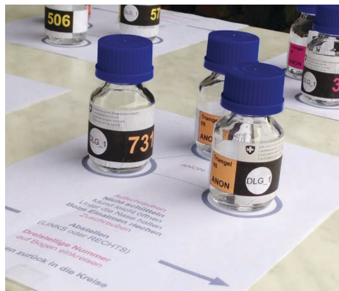
Fig. 2: Triangle test series: in each case, participants are required to identify the sample which differs from the other two (identical) samples.
