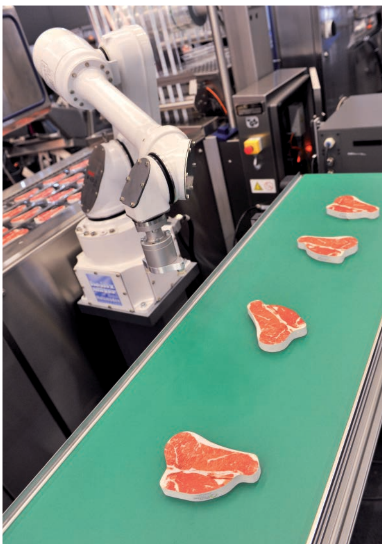
Fig. 8: Articulated robot being used to package meat
