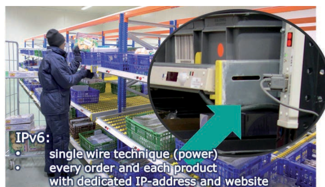
Picture 3: IPv6 smart tags with their own IP address
