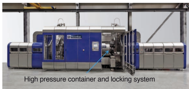
Figure 4: HPP production installation with opened housing
