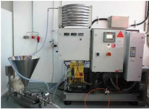
Fig. 1: Ultra-high pressure homogeniser for producing fat-reduced emulsions and functionalisation of ingredients
