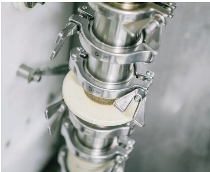
Figure 12: Treatment cell of an industrial PEF system for liquids
