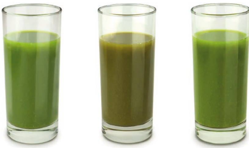
Figure 7: Colour difference of untreated (left), thermally (centre) and PEF-treated green smoothie (right)
