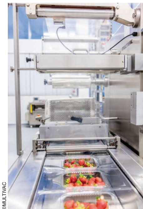
Figure 5: Deep drawing packaging machine and tray sealer each with FreshSAFE application
