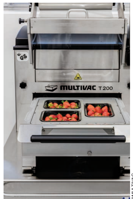
Figure 5: Deep drawing packaging machine and tray sealer each with FreshSAFE application
