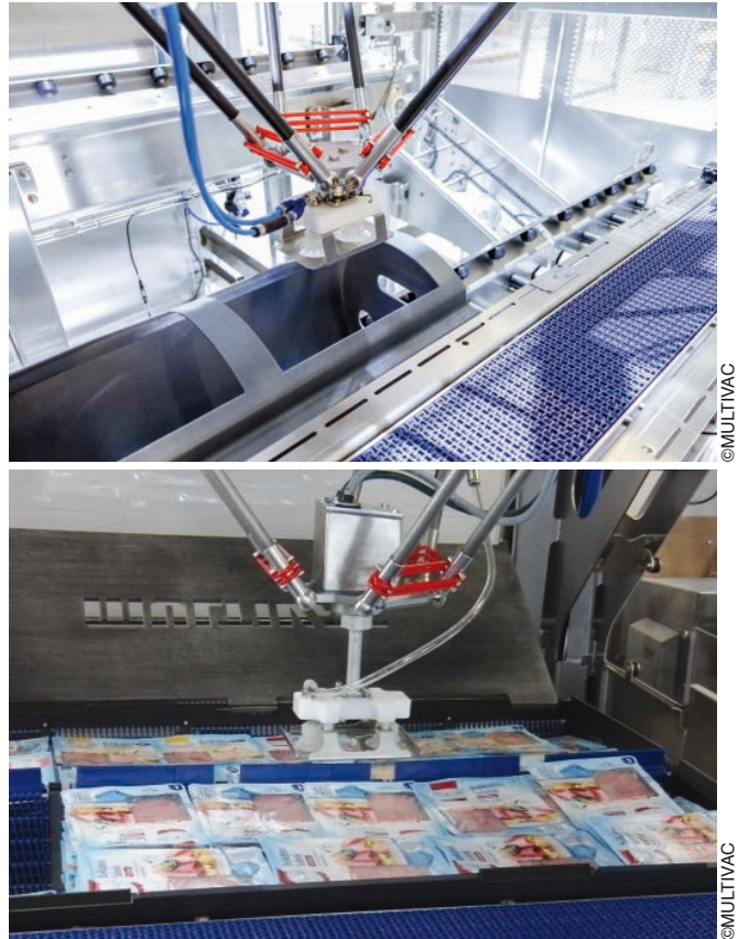
Figure 4: Example of automatic loading of the HPP loading baskets
